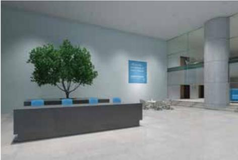
Monotonous lighting that does not take the spatial context into account ignores the perception hierarchies offered by the architecture and makes orientation more difficult for users. It also requires more energy to generate a comparable impression of brightness.
